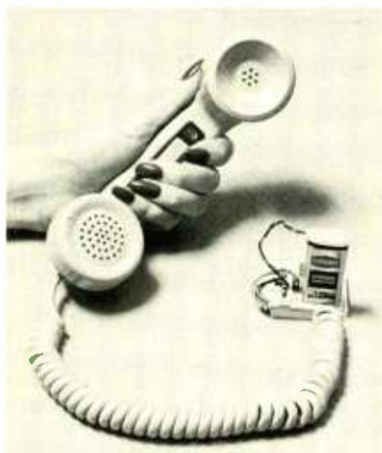
FIG. 1—ONE-STATION INTERCOM is powered by a 9-volt transistor battery and has an LED status indicator.
