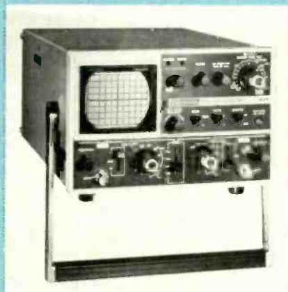
DUAL-TRACE oscilloscope, with bandwidth 15 MHz or more, is needed for VCR troubleshooting and adjustments.
