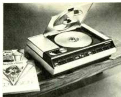
MAGNAVISON PLAYER with the lid up. The unit cannot be turned on until the lid is closed.
